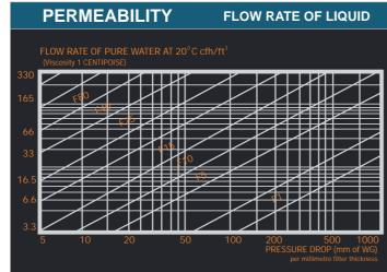
The permeability coefficient of flamingo sintered bronze filter elements can be calculated using the following formula (Darcy)
